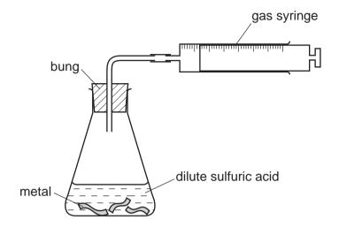
The volume of hydrogen gas collected after one minute was measured.
